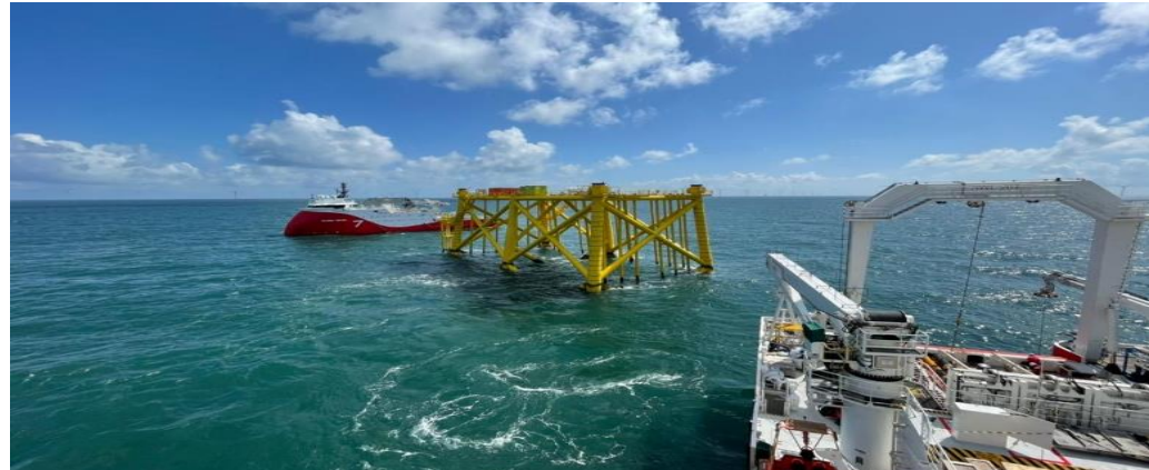
Hornsea II: Seaway 7 'Duo' in action at the OSS
