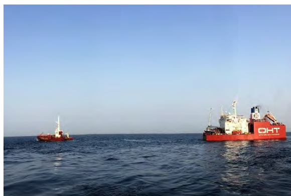
Figure 2 - HTV submerged, ready to take onboard cargo:
