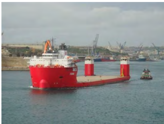
Figure 5 - Dockwise Forte – a custom-built semi-submersible vessel
