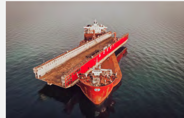
Hawk with a floating dock measuring 180 x 37m from Abu Dhabi to Brest.
